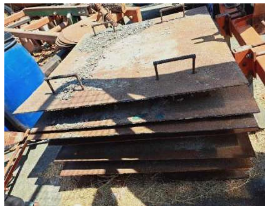
Fabricated Steel Covers
